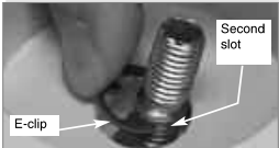
Fig. 5b: Snap e-clip all the way onto shaft above mount (shown partially attached).
