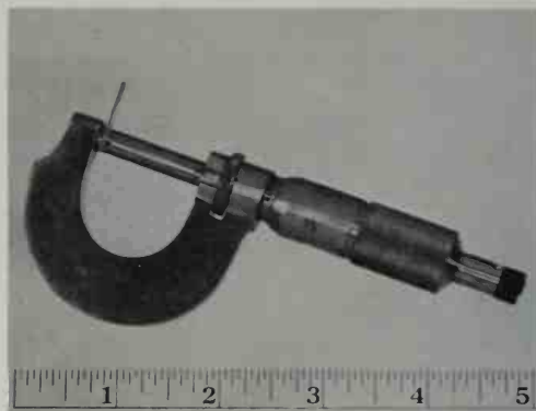
3-10. A micrometer caliper (above). Very small lengths, such as the thickness of a piece of paper, can be measured with this instrument. The basic part of this device, as shown in the simplified version sketched below, is a screw. Note the scale around the barrel, corresponding to the disc below, which enables us to measure a fraction of a turn. How does a screw help us to measure a small distance accurately?
