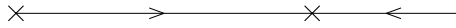
Fig. 32.2. The phase portrait for either species in isolation; the left stationary point represents a population of zero, the right-hand one the equilibrium value ( x = A/a or y = B/d ).
